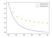
The error is defined as the sum of the squares of the differences between the ordinates of the measured points and that of the computed ones (here error  $\simeq 6.38$ )
