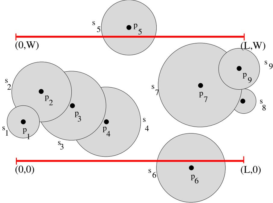
Figure 4: An example of a barrier coverage problem with two parallel barriers
