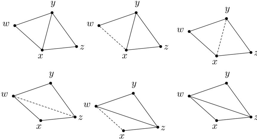
**Fig. 3** Flipping edge  $xy$  to  $wz$ .
