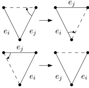
Fig. 9 Exchanging the labels of  $e_i$  and  $e_j$  using three edge rotations.
