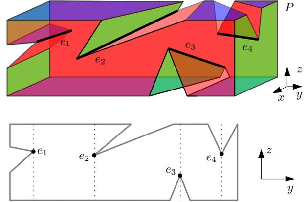
Figure 3: Top: An left edge  $e_1$ , a right edge  $e_2$ , a lower edge  $e_3$ , and an upper edge  $e_4$  in a polyhedron  $P$ . Bottom: The cross-section of the polyhedron  $P$  with a plane parallel to the  $yz$ -plane, which is stabbed by edges  $e_1, \dots, e_4$ . Dotted lines indicate the vertical lines passing through the the stabbing points of  $e_1, \dots, e_4$ .
